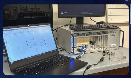
Hardware-in-the-loop (HIL) testing is commonly used in the aerospace industry. The attitude, dynamics, and controls subsystem (ADCS) is one of the most common subsystems to be tested using HIL. The PolySim ADCS lab wants to implement HIL testing for future projects and student development. For this, a HIL test system was created using a Speedgoat Performance Machine and a Raspberry Pi. Three tests were conducted to ensure the test system was set up properly.
