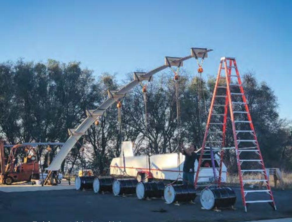
The infamous static load test with the wing at 4gs and 16 feet of deflection prior to failure.
