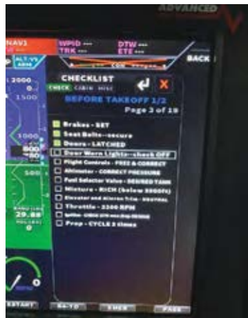
Many electronic flight instrument systems allow the creation of a checklist customized to your airplane. Strict adherence to the checklist will minimize the risk during the stress of a first flight.
