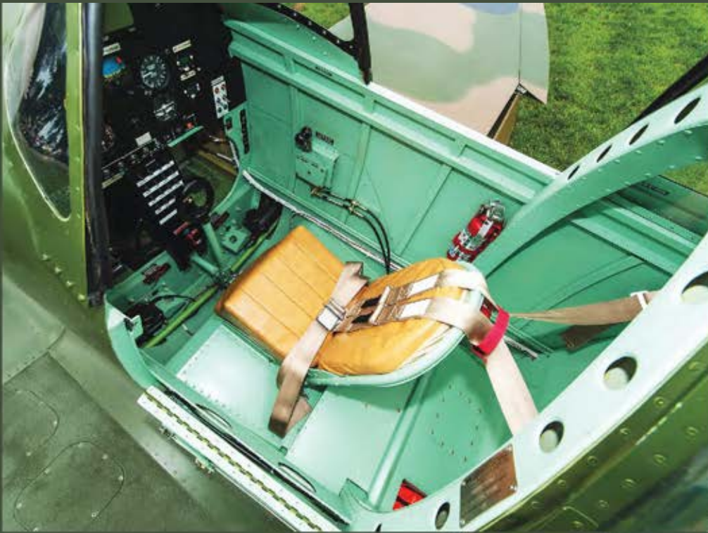
From the Malcolm hood canopy to the iconic spade grip, the cockpit goes a long way toward providing the immersive Spitfire experience.
