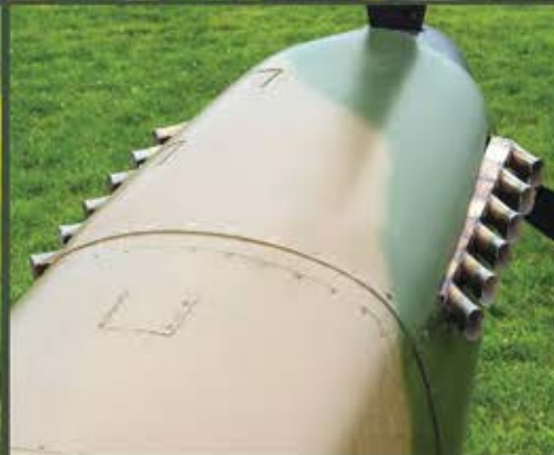
The custom manifold and exhaust stacks lend authenticity to Bob's replica.
