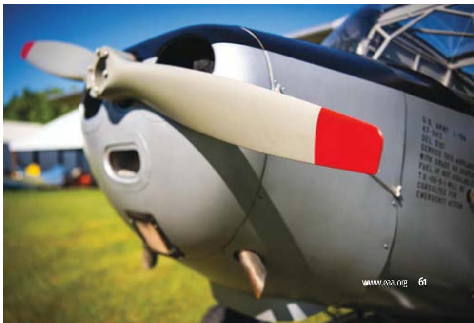
Below: The L-16, which was produced after the L-3, offered a cowled engine compartment and slightly higher horsepower.
