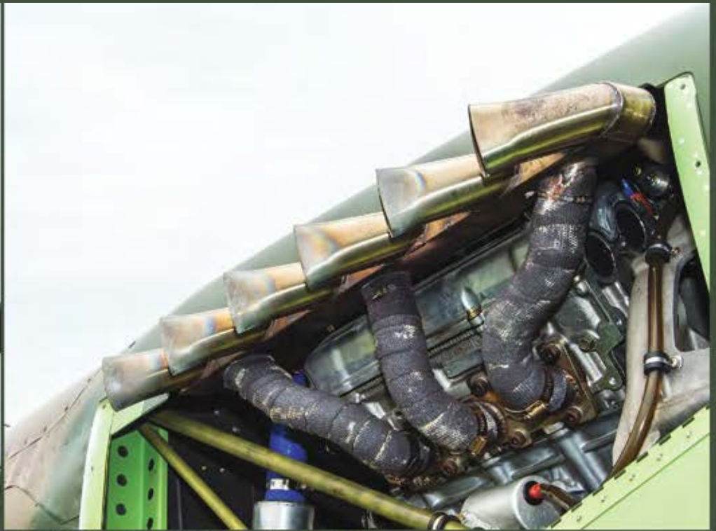
The custom manifold and exhaust stacks lend authenticity to Bob's replica.
